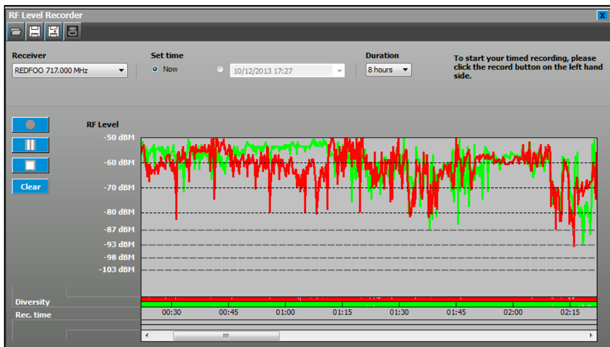
Figure 1 - Example of Radio Microphone Signal Fading – Red and Green traces show signal strength received at the two spaced diversity antennas over approximately two hours of operation.
