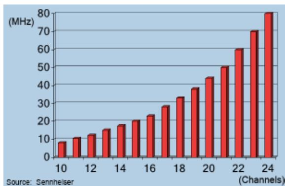
9. The chart above further demonstrates the extent to which Ofcom’s assumptions for how many wireless microphones can fit into an 8 MHz channel are extremely questionable, particularly as they have not taken into account the type of equipment that is likely to be used (high-end analogue equipment). Ofcom must clearly gain a much better understanding of the limits to efficient use of UHF Bands IV and V by wireless microphones and IEMs.
